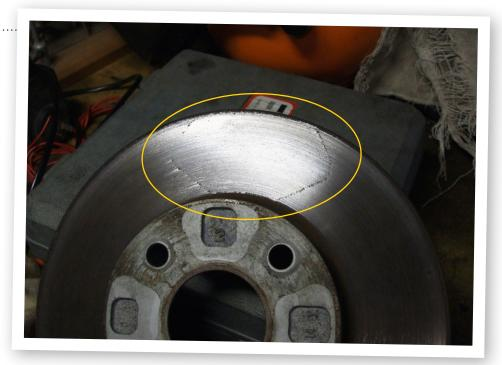
practice not to jam on the hand brake while the brakes are hot (whether after a stint on the track or on a Club run), as this constrains the discs from moving while cooling and can also result in the pads being "welded" to the disc, due to the combination of heat and pressure.
