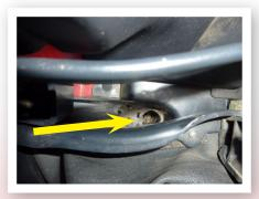
In the NC, the arrangement is much more civilised, and the rectangular draining hole can be seen clearly behind the seatbelt tower, and accessed very easily.
