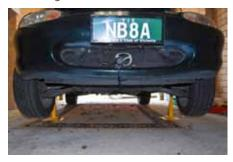
Jack up the car and place it on jack stands. *Note: NEVER get under any car that is only supported by a jack. On most vehicles this is a very dangerous practice ... with the low clearance of an MX-5 it is suicidal!*
