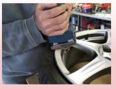
Carefully sand out the damaged areas ...
