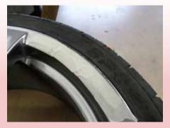
Mask around the damaged area ...
