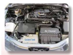
If you have an early NC ('06 to '08), consider replacing your original coolant tank before it fails. There is the possibility the tank could fail while driving and the resulting coolant loss, if not noticed quickly, could lead to overheating and expensive engine damage.
