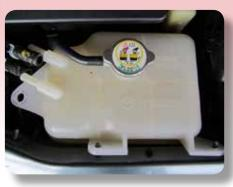
Carefully lift the tank and disconnect the hose underneath, then remove the tank.
