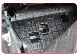
7. The wedge is located on two studs; just pull the wedge away from the floor. The studs are not used for anything - to my knowledge – other than locating the plastic wedge and they need to be trimmed flush with the sound deadening (they will still locate the wedge if you chose to refit it). How you remove the excess material is up to you ... pliers, side cutters, hacksaw, Dremel, grinder or bolt cutters (my choice) are but a few options.
