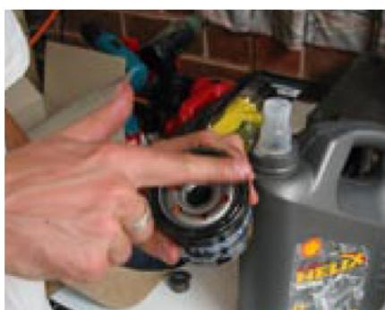
*Pour a little oil into the filter and then rub some of it on to the black rubber seal.*
