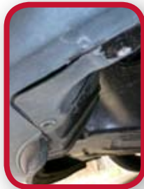
Bolts securing passenger-side splash panel
