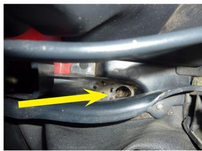
In the NC, the arrangement is much more civilised, and the rectangular draining hole can be seen clearly behind the seatbelt tower, and accessed very easily.
