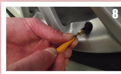
8 Remove the injection hose from the valve. Reinsert the valve core into the valve, and turn it clockwise to install it.
