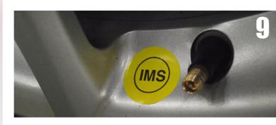
9 Attach the sticker that indicates completion of the tyre repair on a flat outer surface of the repaired tyre.
