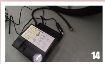
14 Once the tyre is inflated to the correct pressure, switch off the compressor and remove the compressor hose from the tyre valve.
