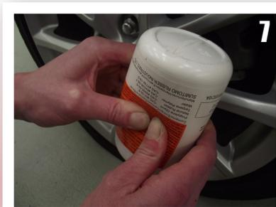
7 Hold the bottom of the bottle upright, squeeze bottle with your hands, and inject all of the tyre sealant into the tyre.
