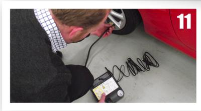
11 Attach the compressor hose to the valve.
