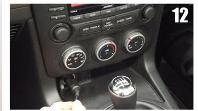
12 Insert the compressor plug into the interior accessory socket and turn the ignition switch to the ACC position.
