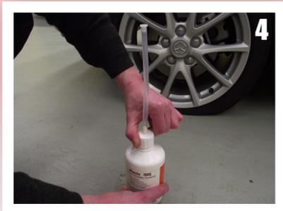
4 Remove cap from the bottle, and screw on the injection hose with the bottle's inner cap left on to break the inner cap.
