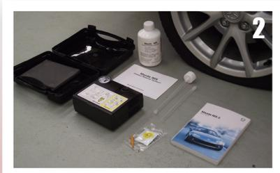
2 Remove emergency flat tyre repair kit.
