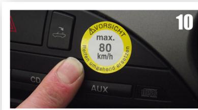
10 Attach the vehicle speed restriction sticker in a place where the driver can see it easily.
