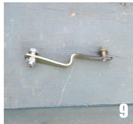
My bracket (#9) is just a piece of bent metal but it does the job. If you have a hammer, vice and drill you can knock something up in a couple of minutes. Obviously the length and shape of the bracket will vary, depending on where you've chosen to mount it. I also took an angle grinder to the bolt supplied with the horn, as I found it was too long.
