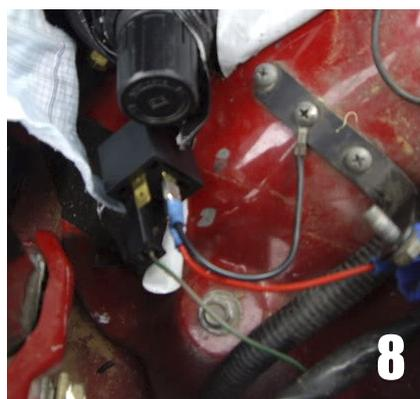
You'll notice I've followed convention and used red wire for the 12V, so I'll use black for the earth (#8). Again, make a wire with a terminal clip and attach it to terminal 85 on the relay. The other end of the wire will have a spade connector from your terminal kit, and this can be attached to
