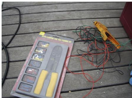
Using your terminal kit, make yourself a wire to run from the 12V source to terminal 30 on the relay. Your terminal kit will have different sized connectors; make
