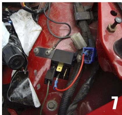
Then make another wire for the earth/ chassis connection at the relay.
