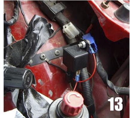
All that's left to do now is cross your fingers and give it a test beep! Remember that the car ignition will need to be switched to the on position when you do this, as the blue plug is not constantly live. Hopefully when you hit the horn button you'll be greeted with a healthy blast of noise. It's not ear-splittingly loud, but it is certainly a vast improvement on the standard item.
