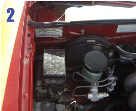
Running a wire from here, with an inline fuse of an appropriate rating (as described in the Stebel literature) would be your best bet.
