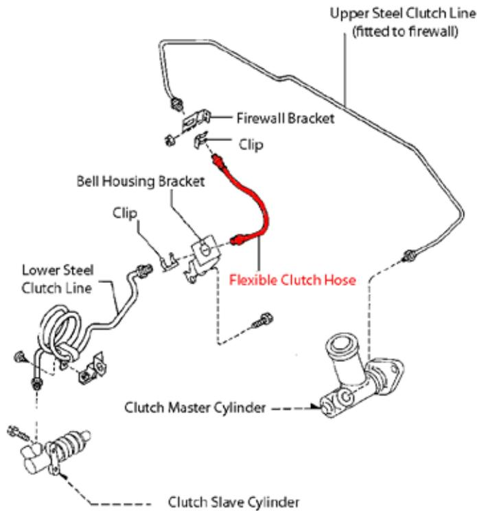
the slave cylinder and the “pig tail” bolt and tighten both (in that order). Fully tighten the bell housing bolt and refit the loom clip to the side of the gearbox. Unless you have miniature hands, don’t attempt to refit the plastic loom clip to the bell housing bracket – we will deal with that later.
