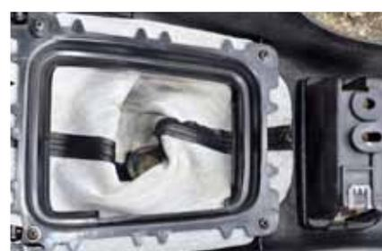
With the console out of the car, turn it over and you will see four Phillips head screws holding a black surround; remove those screws and the surround and you can now remove the shift boot.
