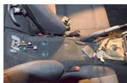
You will see a plastic clip holding that loom to the ashtray area; pop the loom off the console and it is ready to remove. Lift the console from the front clear of the shift lever, and position the boot release and fuel door release levers level with the wider section of the slot they are in and slide the console forward.
