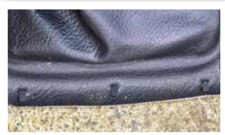
The shift boot is held on to its frame by little black metal clips (spikes?). Remove the old boot from the spikes then fit the new boot's pre-cut slots to the spikes.
