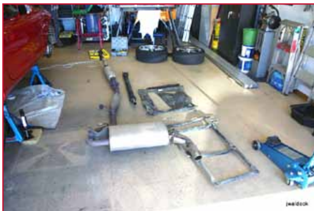
Braces, exhaust and tail shaft removed
