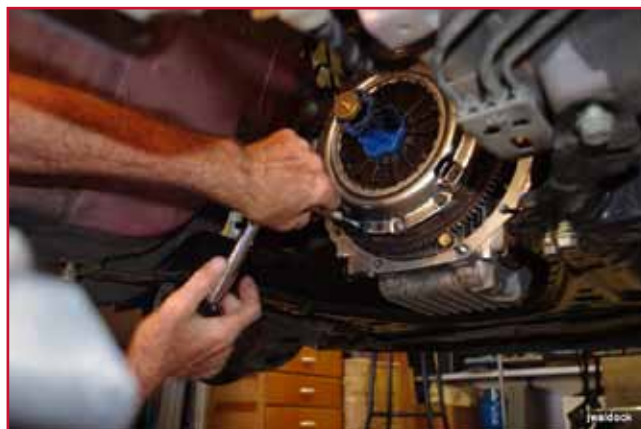
New clutch and bellhousing, with clutch alignment tool
