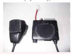
I mount the radio between the seats on the rear bulkhead and the microphone on the passenger side of the transmission
