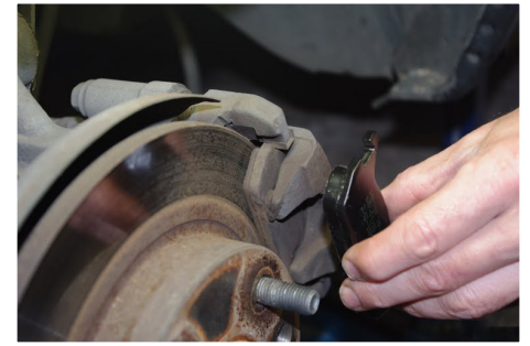
Comparison of new and old brake pad thickness
