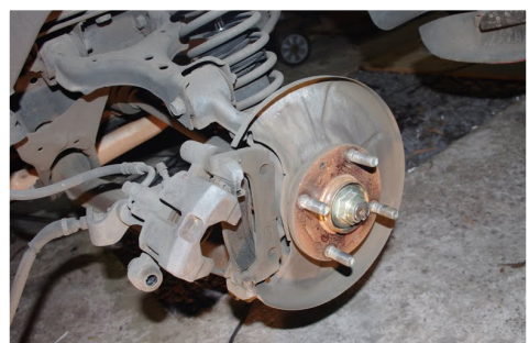
The disc is easily removed before replacing the pads
