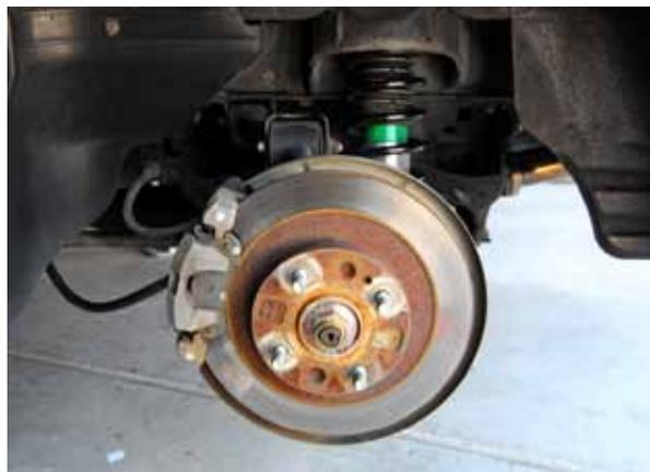
sides of at least one tire to keep the car from rolling. Put the shifter into neutral and release the parking brake. Slightly loosen all the lug nuts on your wheels. Jack up the car one side at a time, placing two jack stands under each door between the notches per factory specs. Before proceeding, give the car a good shake to make sure it's stable. Remove all four wheels.
