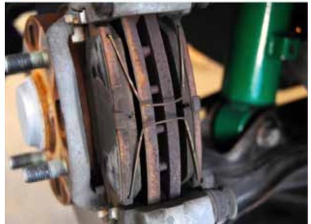
This is a reference photo to show you all of the extra bits associated with the front pads. There are four anti-rattle clips, two U shaped spring pins, and one squealer that clips on the back pad (not pictured). Each front brake pad also has a shim that fits between the pad and the caliper. Performance pads
