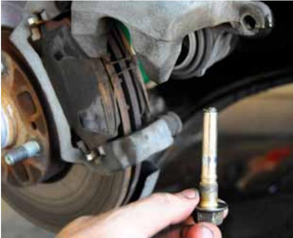
The lower front slider pin (17mm head, I believe) has the highest torque of any bolt you'll be touching in this whole job. You'll probably need a breaker bar to get it free.
