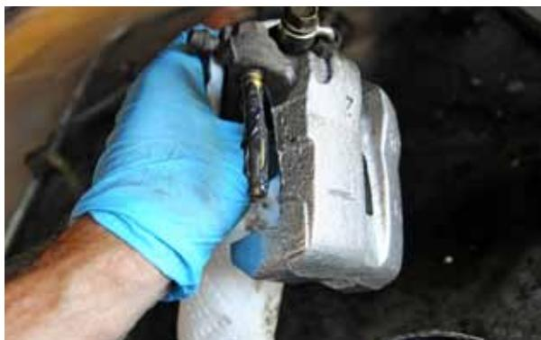
Grease up the top caliper pin. Again, use grease that's meant to deal with brake heat. Then slide the caliper and pin onto the mounting bracket. Rotate the caliper down and partially over the pads. This will allow you to fit the U-shaped spring clips onto the pads without shooting the pads across your shop floor.
