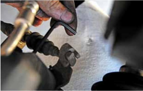
At this point you might be screaming “I can’t get the caliper to fit over my new pads!!!” Well yeah. The new pads are thicker than your old ones, so you’ll have to suck the piston back into the caliper body a bit. You need a 4mm hex key to do this.
