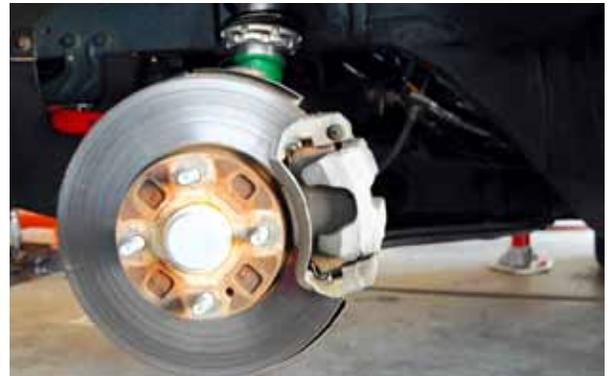
The front brake procedure is exactly the same. Remove pad and rotor.
