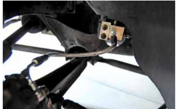
Before mounting the new braided line in place of the rubber line, we have to install the new distribution block.
