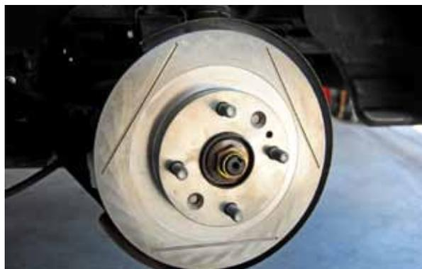
Now is the time to mount your new rotors. Before you do so, don't forget to give them a good cleaning with a spray brake cleaner (Brakleen or something similar). Rotors are usually packed with some grease to keep them from rusting. You want to clean that grease off.
