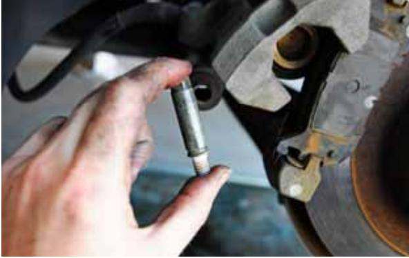
Let's do the rear brakes first. The head of the lower caliper bolt is behind a small plastic cap with a tab on it. This pulls out easily with a pair of pliers. Once the bolt is uncovered, remove it using a 10 mm socket. A low-profile ratchet works well for this one.
