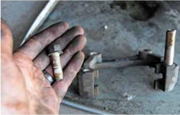
If you're going beyond replacing your pads, you'll need to remove your caliper brackets. They're held in place with two 14 mm head bolts on the back side.
