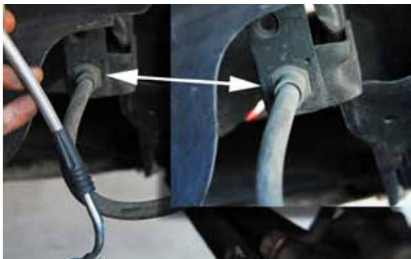
The left side is somewhat different than the right. The flexible hose connects to the end of the hard line crossing under the chassis from the distribution block. Where they meet, they pass through a hole on a tab coming off of the chassis.
