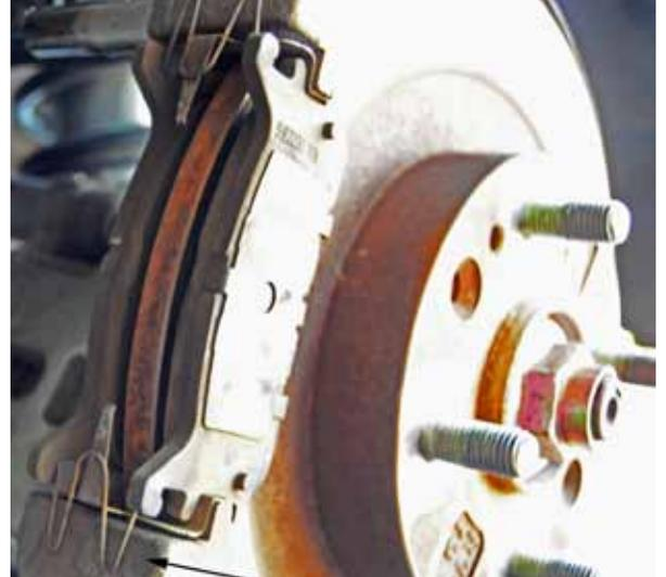
With the caliper out of the way, you can remove the brake pads. This shot shows how the M-shaped tensioner springs fit in place. They can be tricky to get back in, so you'll want to refer to this later when replacing the pads. Also notice the anti-rattle clips on the edges of the caliper. These and the M-springs only come with Mazda factory pads, so don't lose them, you'll need to swap them over to your new pads.
