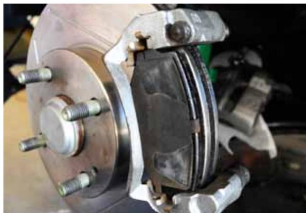
Install the anti-rattle clips on each side of the rotor and then slide the pads in place. This can be a bit
