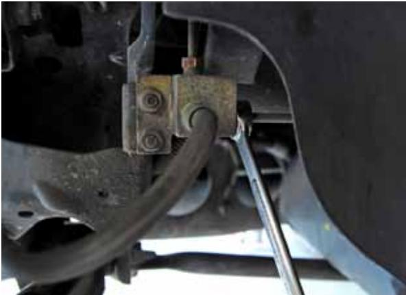
calipers. The factory block has the right rear rubber brake line permanently crimped onto it, so there's no means to attach the new braided line. Hence, it needs to go away.
