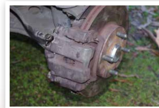
Front caliper with brake line attached
