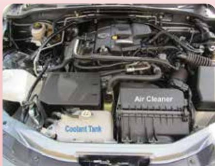
Loosen the two clamps holding the rubber hose between the air cleaner and the inlet manifold.
