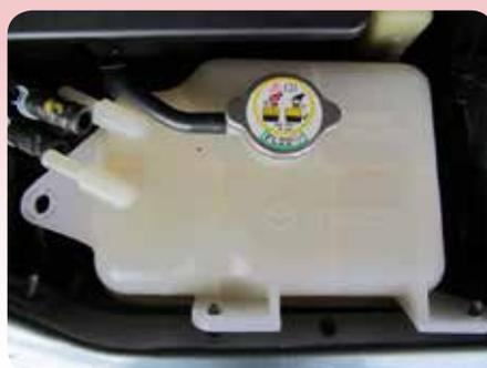
Carefully lift the tank and disconnect the hose underneath, then remove the tank.
