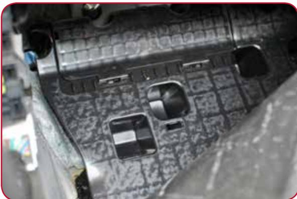
7. The wedge is located on two studs; just pull the wedge away from the floor. The studs are not used for anything – to my knowledge – other than locating the plastic wedge and they need to be trimmed flush with the sound deadening (they will still locate the wedge if you chose to refit it). How you remove the excess material is up to you ... pliers, side cutters, hacksaw, Dremel, grinder or bolt cutters (my choice) are but a few options.
