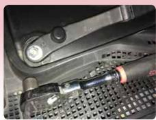
3. Remove the rubber weather seal along the front edge of the plastic cowl cover. The rubber seal is held in place with a number of small plastic T-shaped clips. If you gently stretch the seal lengthwise and lift at the same time, this elongates the hole and allows the seal to come off the T. Once the seal is removed, rotate the clips 90° to remove and reattach them to the rubber seal, ready to be refitted.
