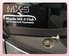
Remove the wiper arms by removing the rubber cap and loosening the 14mm nut a couple of threads; work the arm free from the tapered spline, then remove the nut and arm. Hint: I marked the windscreen at the end of the wiper with a chalk pen to align the wiper.
