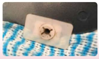
2. Seal the plastic nut with a silicone sealant. Be liberal with the sealant as the cowl cover hides the area and your handiwork won't be seen.
