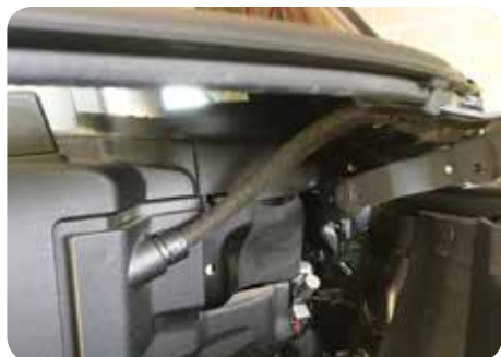
Left and right rear window drains
