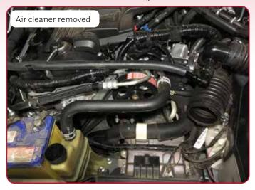
Step 3: Remove the battery box cover, then remove the Neg- and Pos+ leads from the battery. Loosen the hold-down clamps on the battery enough so that the hooks at the bottom can be turned to
