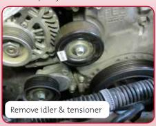
Step 8: Install the new idler pulley and tighten the 10mm bolt to 13-19 N·m (9-14 ft·lbf.) and the tensioner pulley 12mm bolts to 19-25 N·m (15-18 ft·lbf.) Step 9: Install the new belt by twisting the tensioner pulley to the right and slip the new belt on following the diagram below. An extra set of hands - or a method to hold the belt in place – is handy as the belt doesn't want to stay in place until it's tensioned.
