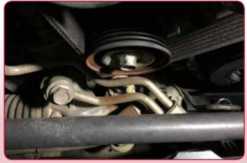
After 170,000km, it was time to replace my belt and both idler and tensioner pulleys were showing signs of wear.
