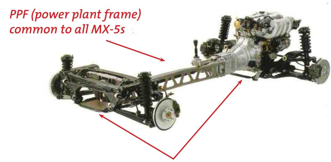
Bracing to rear suspension, under gearbox and between seat belt towers
