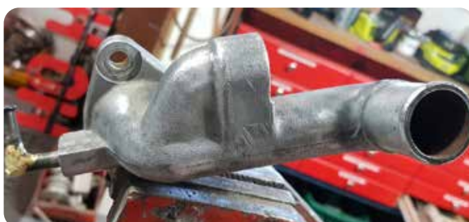
Cooling outlet with rusting corner on steel pipe ... tried repairing it but not confident, so another $260 down the drain!
