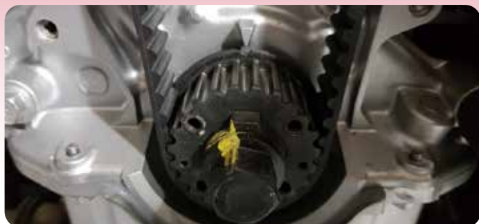
Short nose crank: great care required with fitting up, new bolt and torque (see article mxtra – June 2021)
