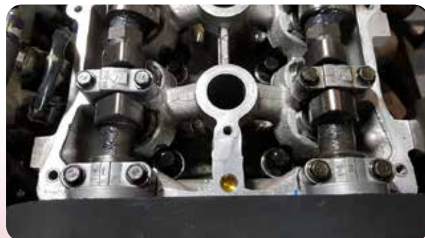
Mis-timed cams: No 1 @ TDC and cams SHOULD be at 9 and 3 o'clock, NOT 12 o'clock!
