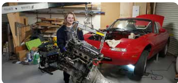
A helper is really useful when removing engine/gearbox or putting back in – just to guide the gearbox
