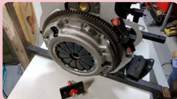
New clutch. Home-made crank lock to allow tightening of crank nose bolt plus clutch bolts
