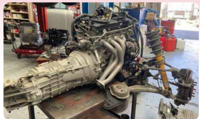
Old 2.0 engine and subframe removed from the car
