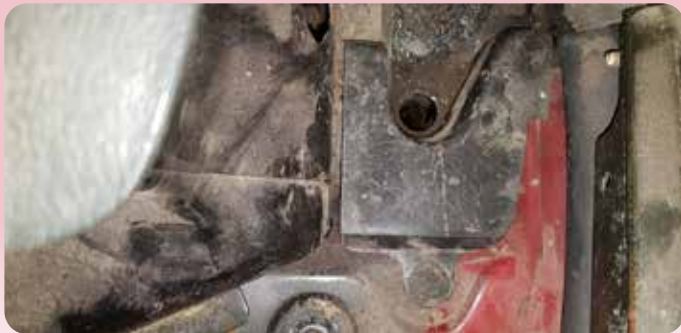
The drain hole behind the seat belt tower
