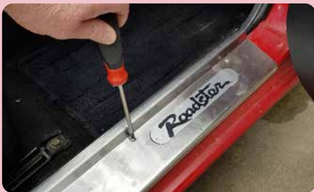
Door sill removal
