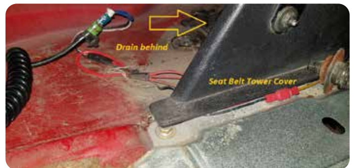
Another view to help locate the drain tube
