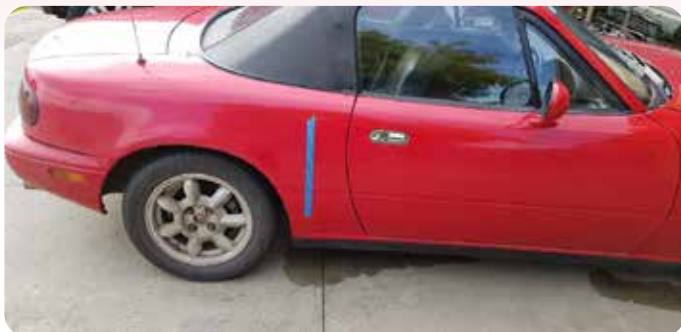
The blue tape in the photo above shows the approximate position of the drain channel. Note the puddle underneath!
