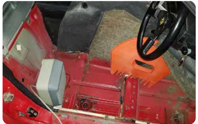
Fan heater, drying the front floor
