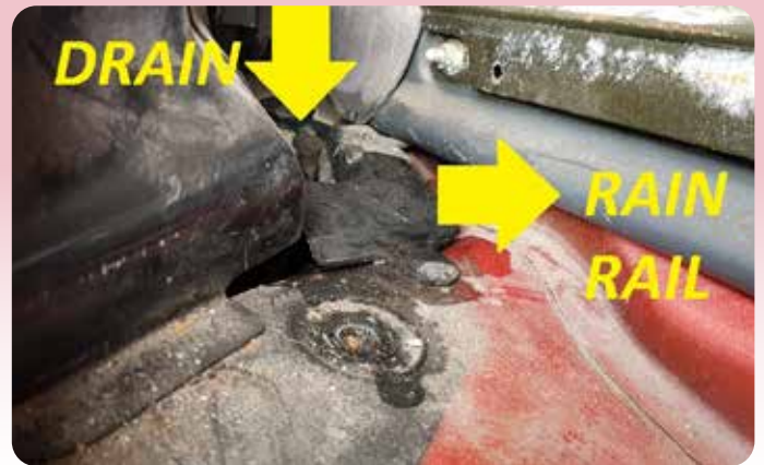
Rain rail and drain
