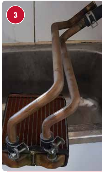
Above: Heater core and outlet copper hoses after pressure testing. Note that the rubber connector tubes may be over 30 years old and were still in good condition
