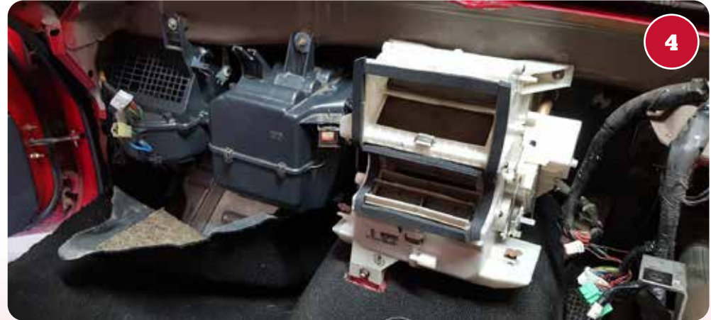
This is what the back of the firewall looks like once the dash is removed: the box on extreme left is blower and selector for fresh or recirc air; the box in centre is the A/C unit, the white box on right is the heater unit. See plastic cover plate on extreme right of this box with wiring harness beside it and clutch pedal obscured. Removing this cover plate gives access to heater core and pipes
