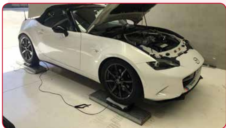
^ Each individual coilover is set up taking into account the driver's weight
