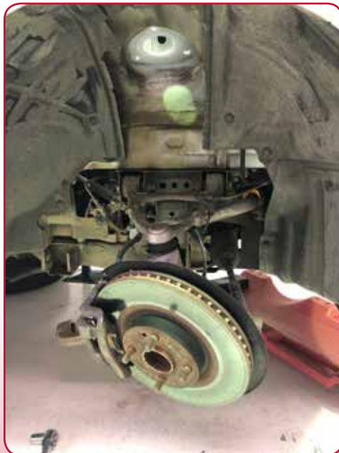
^ Front and rear suspension. The grey springs are the original Whiteline springs with the original Mazda shocks
