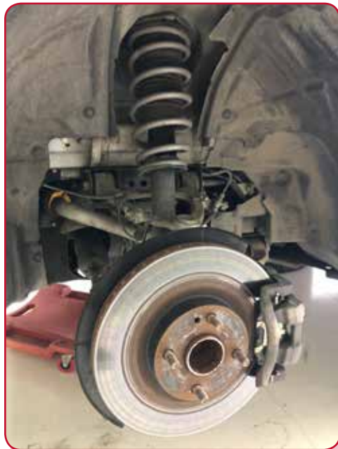
^ Front and rear suspension. The grey springs are the original Whiteline springs with the original Mazda shocks
