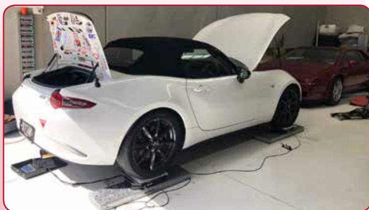
^ Each individual coilover is set up taking into account the driver's weight
