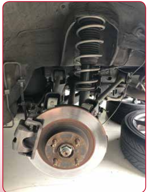
^ Front and rear suspension. The grey springs are the original Whiteline springs with the original Mazda shocks
